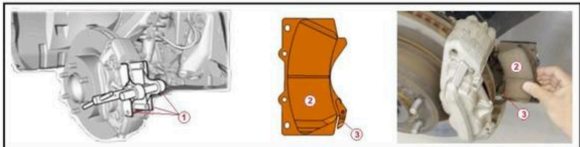
Figure 5. Brake Pad Installation
